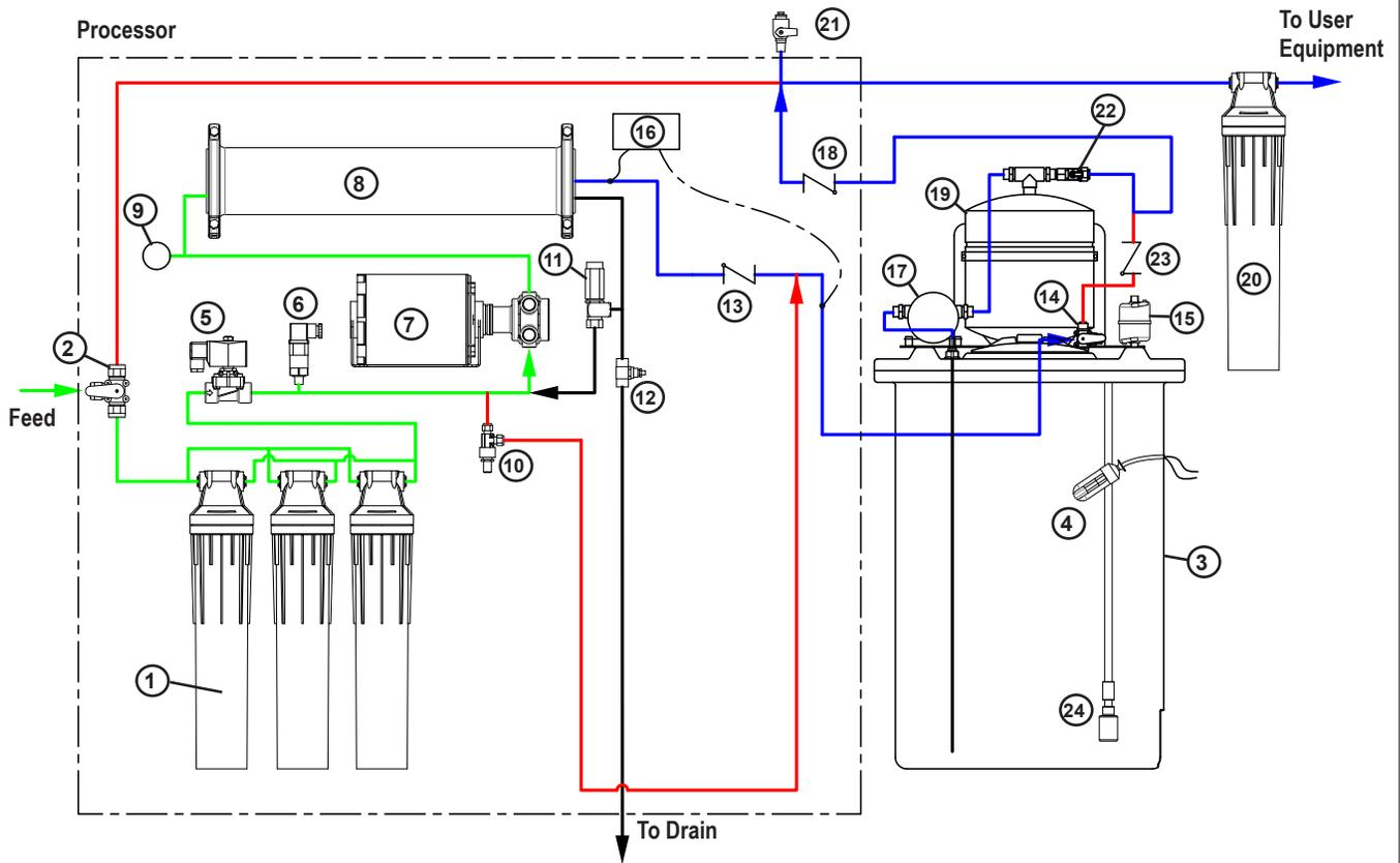
stream exiting the Membrane (8). The Water Quality Monitor is battery powered with two AA batteries. It will automatically shut-off after 30 seconds.
