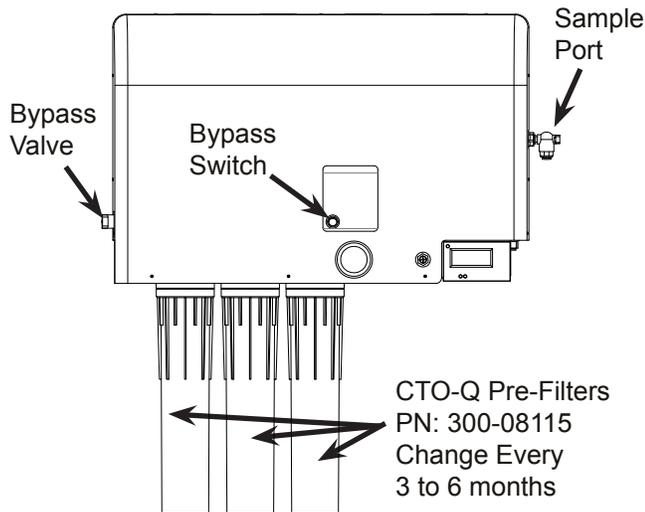
Normally, the most frequent routine maintenance required on the system is periodic replacement of the carbon/sediment pre-filters and the optional post-treatment cartridge. The CTO-Q cartridges should be changed every 1 month to 2 months, depending on water usage. In areas with high levels of sediment and other contaminants the CTO-Q cartridges may require more frequent changes.
