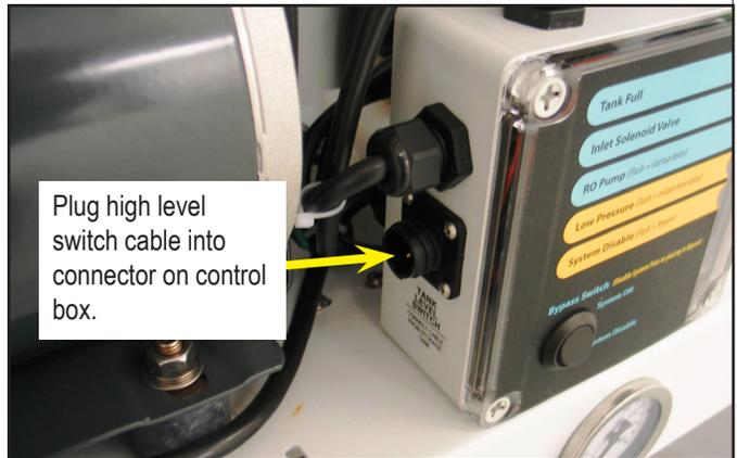
High Level Switch Cable Connection
