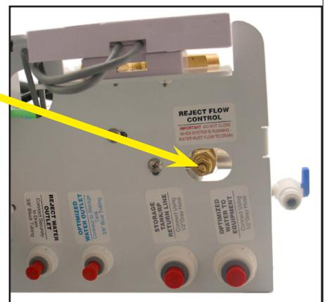
Reject Flow Control (Adjust with Blend Valve Closed) – Never close it nor limit Reject flow to less than Permeate flow!
