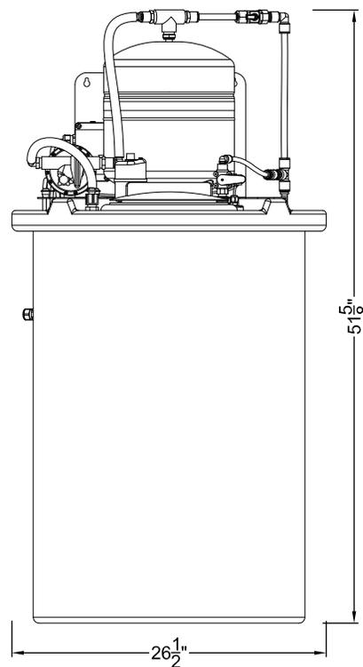
**IMPORTANT - ALLOW A MINIMUM OF 24" IN FRONT OF THE PROCESSOR FOR MAINTENANCE AND SERVICE. DO NOT MOUNT SYSTEM ABOVE THE CEILING OR IN A LOCATION THAT IS NOT EASILY ACCESSIBLE. WHEN THE 50 GAL. TANK ASSEMBLY IS FULL OF OPTIMIZED WATER IT WILL WEIGH 450 LBS (THE 175 GAL. TANK, 1500 LBS). ALWAYS LOCATE THE STORAGE TANK WHERE IT CAN BE ACCESSED DURING SERVICE.**
